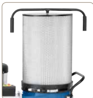
Cartridge filter feature cleaning brushes for effective fine dust removal.
