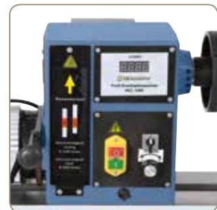
Digital display - as part of standard equipment - ensures comfortable, smooth speed setting.
