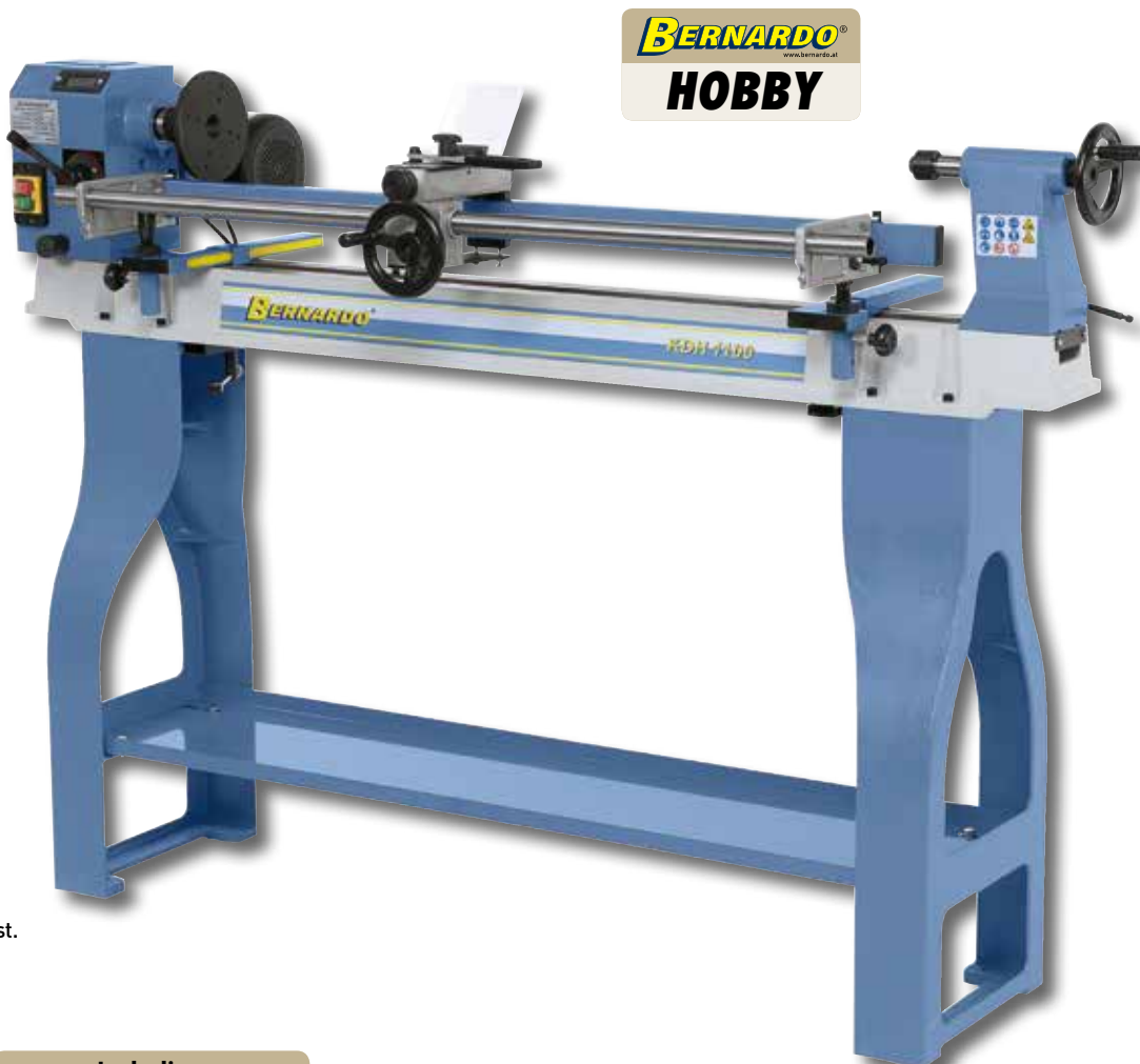
Solid variator drive ensures effective speed transmission from motor to spindle.
