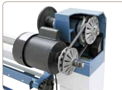
The solid variator-drive guarantees ideal power transmission
