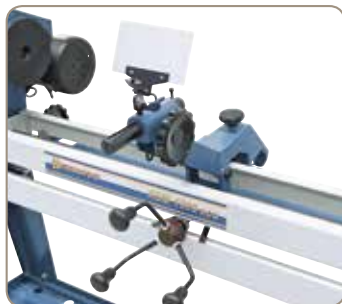
Part of the standard equipment is a copying device for efficient copying of original parts or templates.
