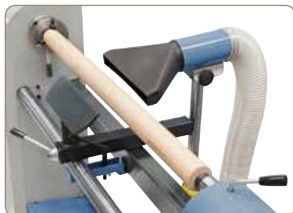
The optionally available dust extractor allows for clean working conditions.
