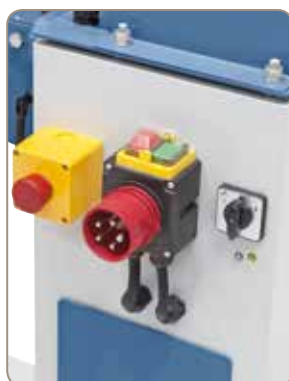
Emergency-off button and rotation switch on machine side.
