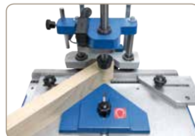
Maximum clearance of 100 mm, maximum milling depth 50 mm (KNF 2 P).
