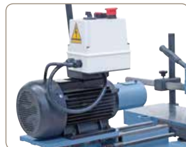
Powerful 2-step motor ensures optimal performance.
